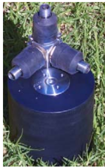
Photo above: Data capture module 24-bit A/D delta-sigma sampling up to 50 KHz
